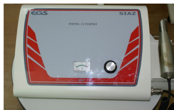
Figure 4. SIAZ-EGS Med-Stomo low-frequency ultrasound physiotherapy device
